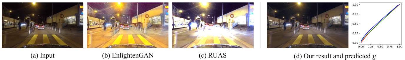
Fig. 12. Enhancement results on Nighttime Driving [97]. Our model automatically finds that the input is bright enough and thus decides not to adjust the illumination, which prevents over-exposure.
